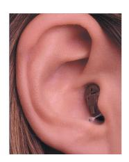
Custom In-the-Ear hearing instruments are used for mild to severe hearing loss. Custom instruments sit entirely within the ear and are fitted individually based on an impression of the wearer's ear. The picture illustrates the range of styles from the CIC "Completely-in-the Canal" (right) which fits completely in the ear canal to the full-shell hearing instrument, which completely fills the bowl of the ear.
